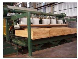
Stacker with automatic veneer grading.
