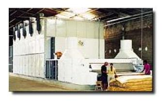
Automatic screen tracking and tensioning keeps it within a fixed side displacement and constant tensioning, results in a longer life. It has a safety device that stops the screen, in case of an excessive side displacement or lack of compressed air.
