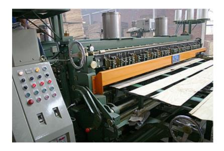
Automatic Veneer Core Composer is eqquipped with thickness detetor, defect clipper, string and glue applicators, clipper for full size veneer and automatic stacker.
